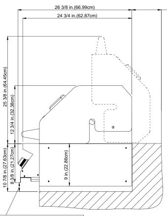
A minimum of 7.875 in.(20.00cm) is required between the back of the grill and any non-combustible material. A minimum of 24 in.(60.96cm)is required between the back of the grill and any combustible material.
